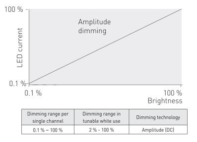
LL50iC-DA-100-1200 LED driver implements amplitude dimming technology across whole dimming range. Amplitude dimming offers the best available technology for dimming the light output in an accurate and flicker-free way to ensure high quality lighting in even the most demanding situations such as camera recording applications. Amplitude dimming technology complies with IEEE 1789-2015 recommendations of current modulation to mitigate health risks to viewers.
