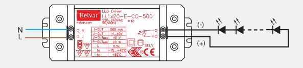
Note: Not suitable for load side switching operation.
