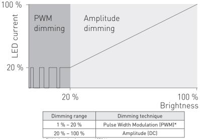
PWM dimming frequency 1250 Hz
