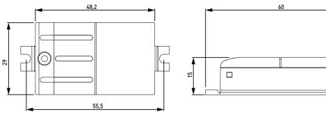
• The mounting tabs can be removed in case they are not needed.
