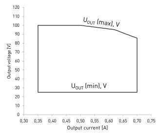
Note: Dimming between 1 % - 100 % per channel possible across the whole operating window
