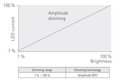
LL80HE-DA-150-850 LED driver implements amplitude dimming technology across whole dimming range. Amplitude dimming offers the best available technology for dimming the light output in an accurate and flicker-free way to ensure high quality lighting in even the most demanding situations such as camera recording applications. Amplitude dimming technology complies with IEEE 1789-2015 recommendations of current modulation to mitigate health risks to viewers.
