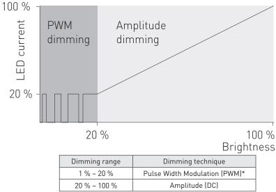
PWM dimming frequency 800 Hz
