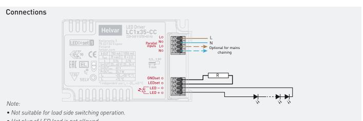
• Hot plug of LED load is not allowed.
