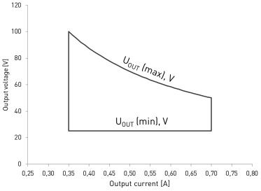
Note: Dimming between 1 % - 100 % per channel possible across the whole operating window
